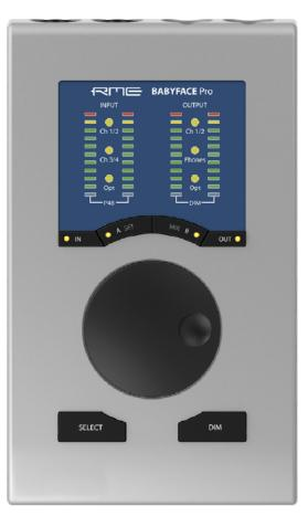
The button **DIM** is also used for **Recall**, to load a specific listening volume for the Main Out that can be defined in TotalMix FX. Pushing the knob SET for 2 seconds when OUT is selected stores the current setting. If the volume (output level) had been changed pressing DIM for two seconds will restore the former value.
