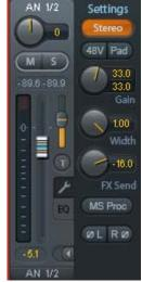
**Loopback.** Sends the output data to the driver as record data. The corresponding submix can be recorded then. This channel's hardware input sends its data only to TotalMix, no longer to the recording software.
