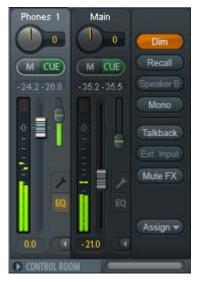
**Speaker B.** Switches audio from Main Out to Main Out B. The faders of the channels Main and Speaker B can be ganged via Link. Via *Options / Key Commands* switching to Speaker B can also be controlled by the unit's **OUT**, **A**, **B** and **DIM** button.
