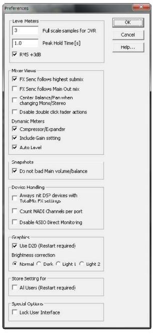
Brightness correction. Set TotalMix FX screen brightness to your taste, matching the monitor setting or the environment.
