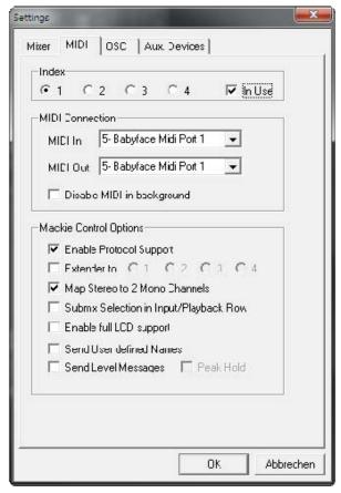
Send Level Messages. Activates the transmission of the level meter data. Peak Hold activates the peak hold function as set up for the TotalMix level meters in the preferences.
