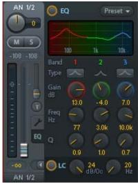
The frequency graphics give a precise overview of the filter results. Overlapping filters influence each other. This can be used to achieve more than 20 dB amplitude, or to generate difficult frequency response optimizations.
