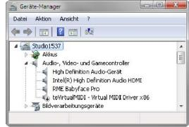
Windows does not support USB Audio 2.0 directly. The Babyface Pro will be detected when in CC mode, but automatic driver installation will fail.
