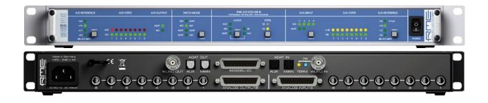
The ADI-8 DS Mk III is a highly flexible 8-channel AD/DA converter and digital to digital format converter with an unrivalled bunch of features. The device combines excellent analog circuit design with outstanding low latency AD/DA converter chips. Along with SteadyClock, the QS offers AD and DA conversion of the highest quality, redefining the reference class of analog/digital converters.
