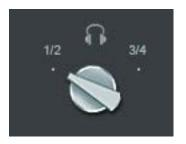
4. Turn zero latency hardware monitoring ON and OFF
