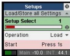
The Fireface UFX can store and load its current state in 6 different memory slots, called Setups. With this, the Fireface UFX can be used stand-alone after setting it up accordingly, replacing lots of dedicated devices (see chapter 25).
