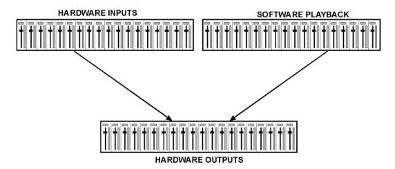
36 channels don't fit on the screen side by side, neither does such an arrangement provide a useful overview. Therefore, the channels have been arranged as known from an *Inline* desk, so that the row *Software Playback* equals the *Tape Return* of a real mixing desk:
