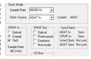
This way, configuring any suitable audio application for digital recording is simple. After selecting the required input, Hammerfall DSP displays the current sample frequency. This parameter can then be changed in the application's audio attributes (or similar) dialog.
