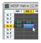
After a mouse click TotalMix sets gains and pans correctly. Of course these settings can also be performed manually. Repeat the last step to remove all routings (*menu Options* ... Off).
