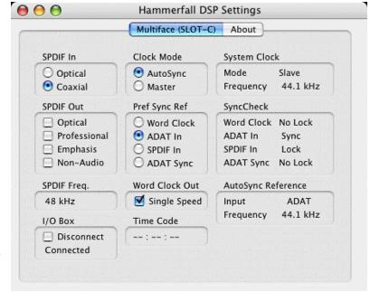
for each input (Word Clock, ADAT, SPDIF), or if there is a valid *and* synchronous signal (Sync). The *AutoSync Reference* display shows the input and frequency of the current sync source.
