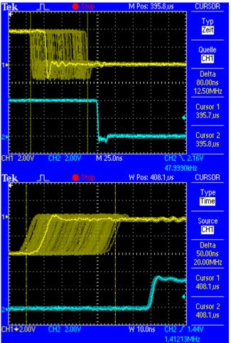
The cleaned and jitter-freed signal can be used as reference clock for any application, without any problem. The signal processed by SteadyClock is of course not only used internally, but is also used to clock the digital outputs ADAT and AES/EBU.
