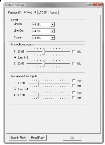
The option **Link** simplifies the setup in case both channels shall have the same setting/values. The current gain is displayed in dB below the fader.
