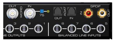
**Word Clock** I/O (BNC): A push switch activates internal termination (75 Ohms). When termination is activated the yellow LED besides the switch lights up.
