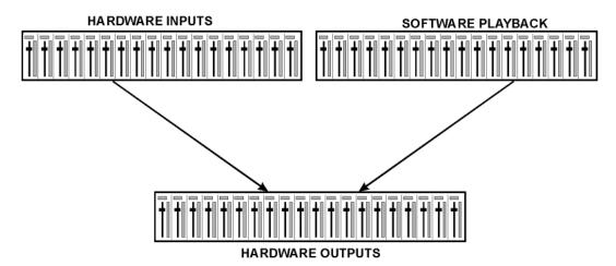
36 channels don't fit on the screen side by side, neither does such an arrangement provide a useful overview. The input channel should be placed above the corresponding output channel. Therefore, the channels have been arranged as known from an *Inline* desk, so that the row *Software Playback* equals the *Tape Return* of a real mixing desk:
