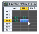
After a mouse click TotalMix sets gains and pans correctly. Of course these settings can also be performed manually. Repeat the last step to remove all routings (*menu Options ... Off*).
