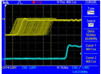
Common interface jitter values in real world applications are below 10 ns, a very good value is less than 2 ns.
