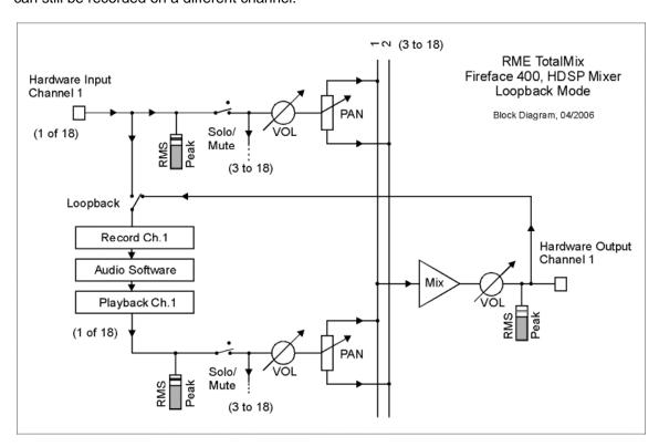
As each of the 18 hardware outputs can be routed to the record software, and none of these hardware inputs get lost, TotalMix offers an overall flexibility and performance not rivalled by any other solution.
