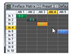
To maintain overview when the window size has been reduced, the left and upper labels are floating. They won't leave the visible area when scrolling.
