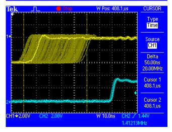
The cleaned and jitter-freed signal can be used as reference clock for any application, without any problem. The signal processed by SteadyClock is of course not only used internally, but also available at the ADI-8 QS' word clock output. It is also used to clock the digital outputs MADI. ADAT and AES/EBU.
