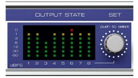
multifunctional device. It is used to set the trim values, the volume, and various options in the Setup menu.
