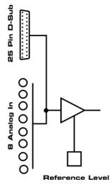
The ADI-8 QS uses a completely symmetrical signal path (including limiter) that guarantees an exceptional sound quality, outstanding low distortion and highest Signal to Noise ratio in all level settings.
