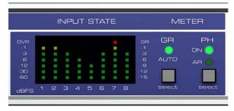
When the Setup menu is active, the according parameter values are displayed in this level meter window.
