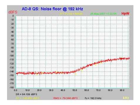
As can be seen in the above picture, the noise floor stays fully unchanged up to 45 kHz. With sample rates up to 96 kHz the noise shaping completely happens outside of the transmission range.
