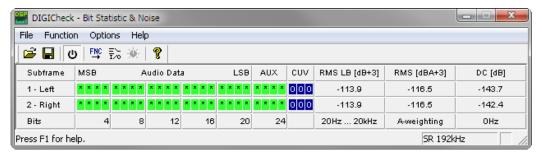
The reason for this behaviour is the noise shaping technology of the analog to digital converters. They move all noise and distortion to the in-audible higher frequency range, above 45 kHz. Therefore the noise is slightly increased in the ultrasound area. High-frequent noise has a high energy. Add the quadrupled bandwidth, and a wideband measurement will show a significant drop in SNR, while the human ear will notice absolutely no change in the audible noise floor.
