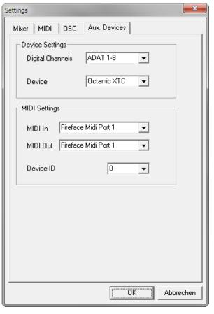
When using more than one OctaMic XTC these must have different Device IDs (configuration is done at the OctaMic XTC). *Aux Devices* supports to set different Device IDs to the 8-channel blocks as well. Storing the setting is done automatically when selecting a Device ID. To check the current assignments toggle the two 8-channel blocks.
