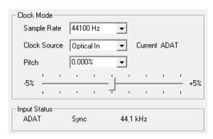
This way, configuring any suitable audio application for digital recording is simple. After selecting the correct input, Fireface 802 displays the current sample frequency. This parameter can then be changed in the application's audio attributes (or similar) dialog.
