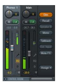
Mono. Mixes left and right channel. Useful to check for mono compatibility and phase problems.
