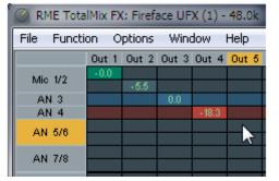
The Matrix not always replaces the mixer view, but it significantly enhances the routing capabilities and - more important - is a brilliant way to get a fast overview of all active routings. It shows you in a glance what's going on. And since the Matrix operates monaural, it is very easy to set up specific routings with specific gains.
