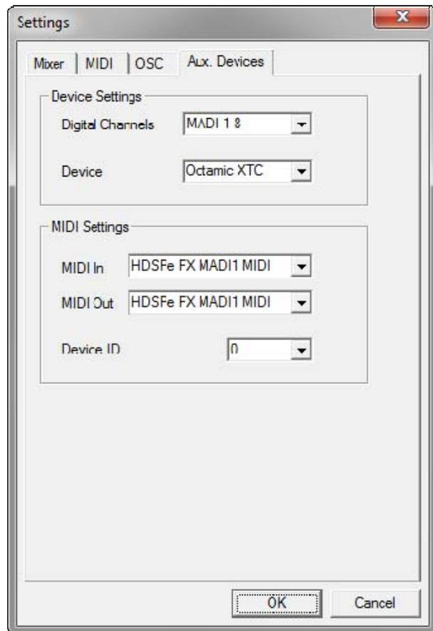
When using more than one OctaMic XTC these must have different Device IDs (configuration is done at the OctaMic XTC). *Aux Devices* supports to set different Device IDs to the 8-channel blocks as well. Storing the setting is done automatically when selecting a Device ID. To check the current assignments select all 8-channel blocks sequentially.
