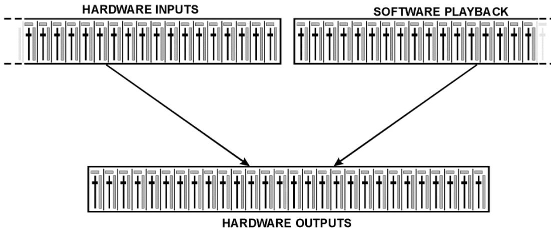
TotalMix can be used in the above view (View Options **2 Row**). However, the default is a vertical alignment in three rows as known from an Inline desk, so that the row *Software Playback* equals the *Tape Return* of a real mixing desk:
