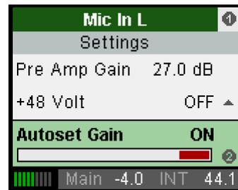
As soon as AutoSet reduces the gain the label AS, shown in the Mic Gain screen, changes its color from black to blue.
