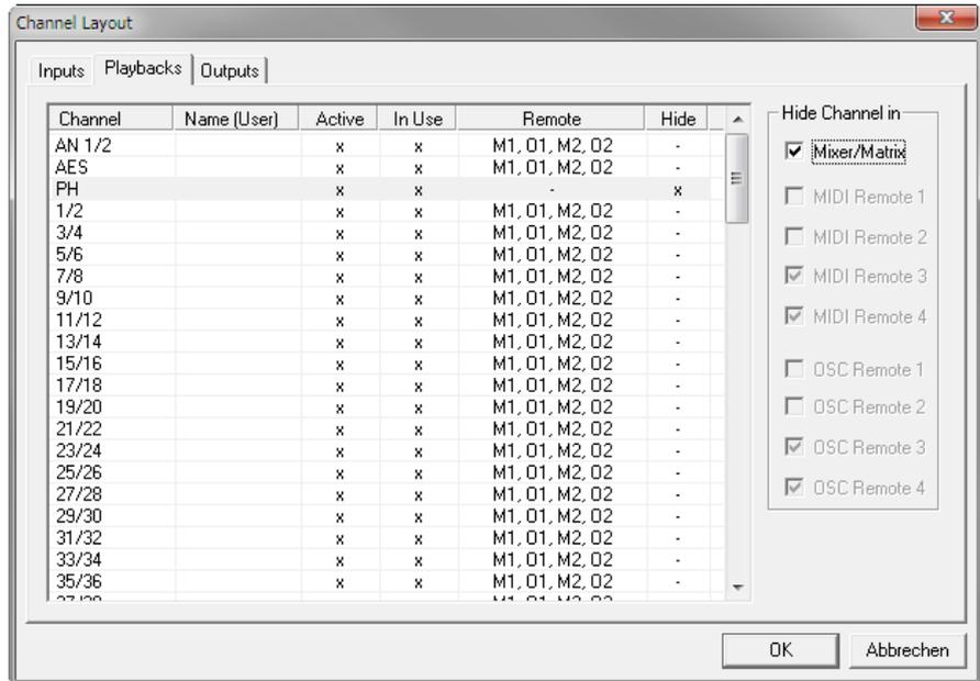
Rows Inputs, Playbacks and Outputs are set up individually by the tabs at the top. *Active* indicates currently available channels. At higher sample rates many MADI channels are no longer active. *In Use* shows which channels are currently used in the mixing process.
