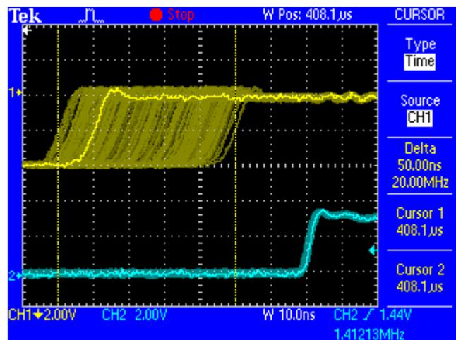
The cleaned and jitter-free signal can be used as reference clock for any application, without any problem. The signal processed by SteadyClock is of course not only used internally, but also available at all outputs.
