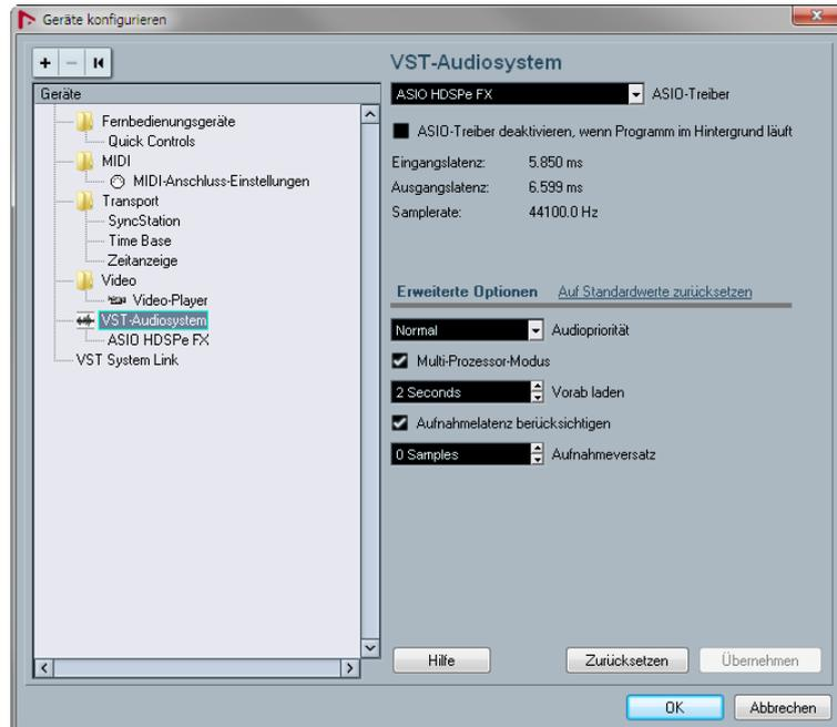
**Note:** When changing the sample rate range between Single, Double and Quad Speed the number of channels presented from the ASIO driver will change too. This may require a reset of the I/O list in the audio software.
