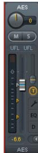
As all channel's routings change simultaneously when Trim is active, this mode basically causes the same behaviour as a trim pot within the input channel, affecting the signal already before the mixer. That's how this function got its name.
