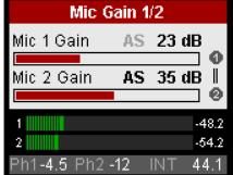
Input 1 to 4 include optional attenuation against too high input levels (PAD, -20 dB). This setting is found in the CHANNEL menu. The 1/4"TRS input within the XLR socket operates like the XLR input, but is 9 dB less sensitive.
