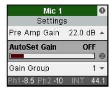
As soon as AutoSet reduces the gain the label AS, shown in the front display, changes its color from black to blue.
