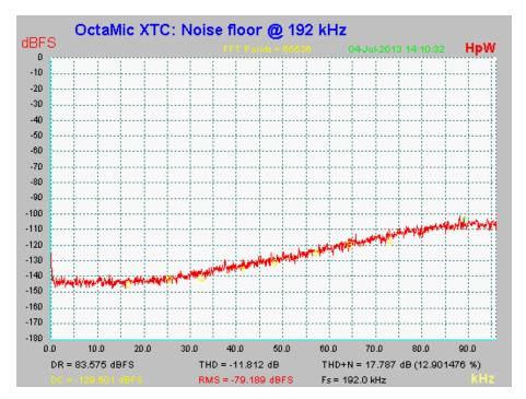
As can be seen in the above picture, the noise floor stays fully unchanged up to 30 kHz. With sample rates up to 96 kHz the noise shaping happens outside of the transmission range.
