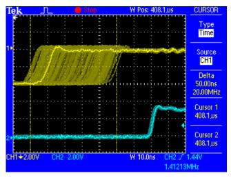
The cleaned and jitter-freed signal can be used as reference clock for any application, without any problem. The signal processed by SteadyClock is of course not only used internally, but also available at the XTC's word clock output. It is also used to clock the digital outputs MADI, ADAT and AES/EBU.
