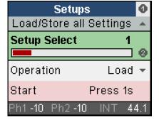
On the Options page several sub-pages exist, therefore a 2 is shown on the right side of those sub-pages. By turning encoder 2 the pages *Clock*, *MIDI Sources*, *General Settings* and *Digital Routing* are shown. The arrow under the 2 indicates that pressing encoder 2 the corresponding page is entered, and settings can be changed then.
