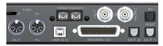
**USB 2.0**: Windows: Firmware update. Mac OS X: Class Compliant audio interface and firmware update. iPad: Class Compliant audio interface via Camera Connection Kit.
