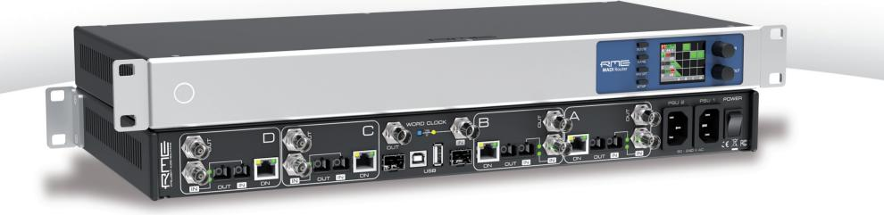
The MADI Router has four groups of three different MADI I/Os each and may be used as a patch bay and format converter between those. Apart from the fully transparent, stream-wise operation between its ports it excels the well-known MADI Bridge by letting users create output signals that combine audio channels from different MADI inputs ("Any-to-any").
