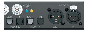
**ADAT2 I/O.** TOSLINK. Standard ADAT optical port, 8 channels. Can also be used as optical SPDIF input and output, if set up accordingly in the Settings dialog.
