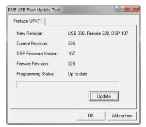
When the update unexpectedly fails (status: failure), the unit's Safety BIOS will be used from the next boot on, the unit stays fully functional. The flash process should then be tried again.
