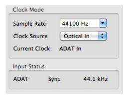
RME's exclusive **SyncCheck** technology (first implemented in the Hammerfall) enables an easy to use check and display of the current clock status. *SyncCheck* indicates whether there is a valid signal (Lock, No Lock) for each input (Word Clock, ADAT, AES), or if there is a valid *and* synchronous signal (Sync). In the field *Clock Mode* the clock reference is shown. See chapter 33.1.
