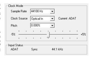
This way, configuring any suitable audio application for digital recording is simple. After selecting the required input, Fireface UC displays the current sample frequency. This parameter can then be changed in the application's audio attributes (or similar) dialog.
