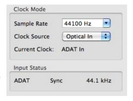
RME's exclusive **SyncCheck** technology (first implemented in the Hammerfall) enables an easy to use check and display of the current clock status. *Input Status* indicates whether there is a valid signal (Lock, No Lock) for each input (Word Clock, ADAT, SPDIF and LTC), or if there is a valid *and* synchronous signal (Sync). In the field *Clock Mode* the clock reference is shown (Current...). See chapter 31.1.
