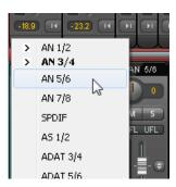
**Trim Gain.** After a click on the double arrow one channel's faders are all synchronized. Instead of changing only a single routing the fader affects all the channel's active routings. For a better overview the faders currently not visible are indicated by orange triangles beside the fader path. When moving the fader the triangles also move to a new position, equalling the faders new settings.
