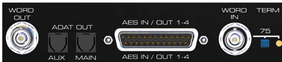
**WORD IN (BNC):** A push switch allows to activate internal termination (75 Ohms).
