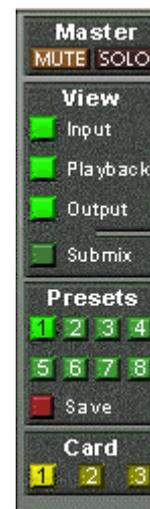
Up to three Hammerfall DSP systems can be used simultaneously. The **Card** buttons switch between the systems (RPM, Digiface, Multiface, HDSP 9652, HDSP 9632). Holding down Ctrl while clicking on button Card2 will open a second window, instead of replacing the current window content.
