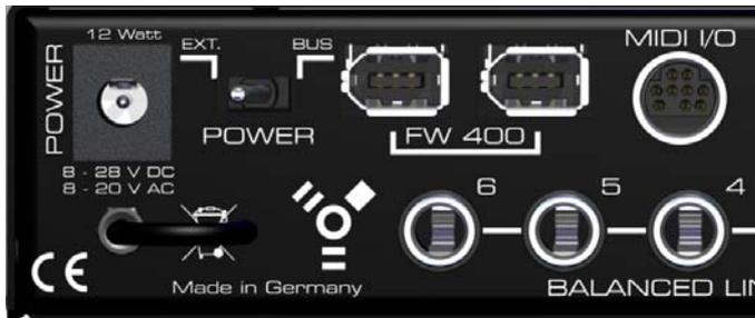
**MIDI I/O**: Provides two MIDI inputs and outputs via the included breakout cable.
