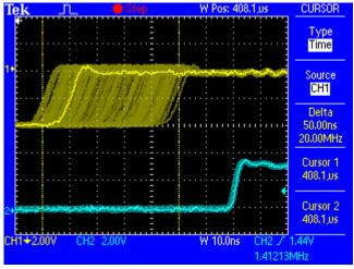
The cleaned and jitter-freed signal can be used as reference clock for any application, without any problem. The signal processed by SteadyClock is of course not only used internally, but also available at the ADI-642's word clock output. It is also used to clock the digital outputs MADI and AES/EBU.
