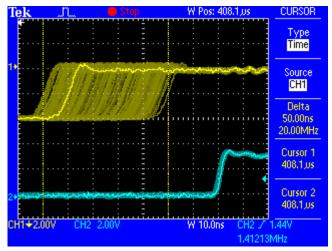
The cleaned and jitter-freed signal can be used as reference clock for any application, without any problem. The signal processed by SteadyClock is of course not only used internally, but also available at the ADI-192 DD's word clock output. It is also used to clock all the digital outputs.
