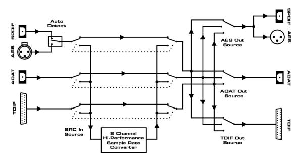
In many input formats, the input signal's effective sample rate stays unclear because of possible sample multiplexing. Therefore the frequency range has to be defined manually via the RANGE button:
